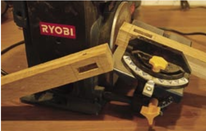
One of the most visible details on the ottoman is the shallow bevel on the leg tops. You could make the cuts using a table saw or miter saw, but I took advantage of a benchtop disc sander that let me fine-tune the bevels as I went.
